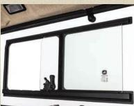
**Rear-Sliding Window**Access the cargo box from the cab, or open to enjoy cross ventilation. Slide window to open partially or fully.
